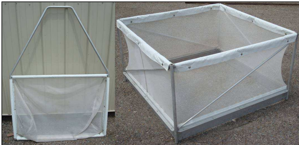
Figure 2. (A) Throw trap sampler deployed in the field for sampling seagrass. (B) Left: Sweep net used to collect organisms captured in the throw trap sampler. Right: Throw trap sampling gear used to sample estuarine habitat types.
