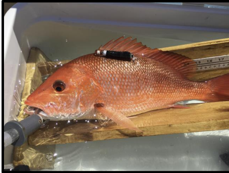
Figure 1.2: Image of the tagging cradle used to measure and tag Red Snapper. This fish was fitted with a Lotek MM-M-8-SO-TP series ultrasonic acoustic transmitter. The gills of fish were submerged in seawater during the measuring and tagging process.
